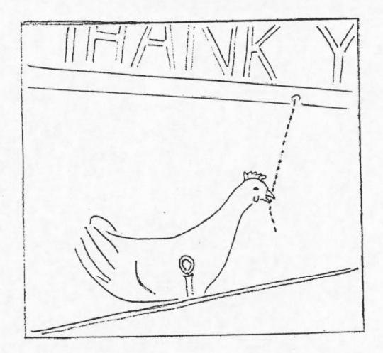
When a visitor puts a dime, or two nickels, into the coin box, the chicken responds to a red signal light by pulling the chain to light the "Thank You" sign.
