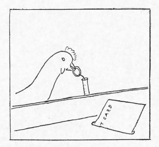
As the "Thank You" sign lights, another red signal lights up to "tell" the chicken to pull the loop to activate the card dispensing mechanism. A card then comes up through the slot to the customer. As the card rises, the feeder rewards the bird for her efforts. The "Thank You" sign lights go out, and the vendor is ready for another customer.
