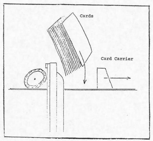
To load cards in the vendor, pull back the carrier and drop the cards in place in it. Be sure, however, that the cards are all the way down in the carrier. If a few cards are allowed to stick up from the pack, they may jam the mechanism.
