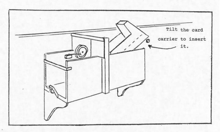
The postcards are held in the vending mechanism in a roller-bearing carrier. If the carrier has been removed for shipment, tilt and lower it so that its rollers rest on the metal track.
