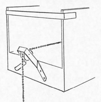
Lead the carrier's chain over the pulley and catch the end of the chain in the hole in the cylindrical weight.
