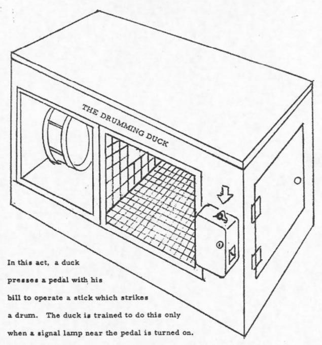
The signal light turns on when the appropriate coin is put into the coin box or when the "test" button is pressed. After 10 or 25 strokes of the stick, depending on the setting of the control knob, the duck is rewarded with a helping of food and the signal light goes off.
